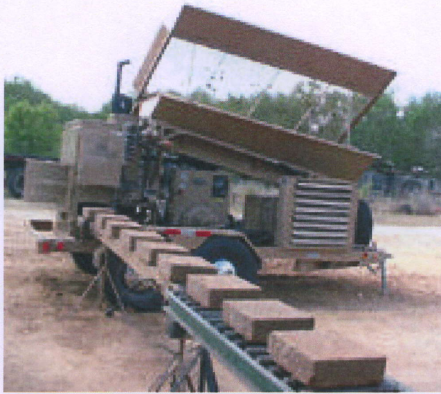
Figure 11. AECT 5000 Series Compressed Soil Block Machine (Photo courtesy of AECT at http://www.webspace4me.net/~fwehman )
