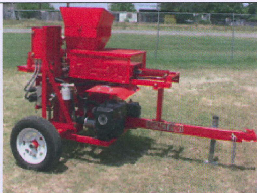
Figure 3. AECT Impact 2001 Compressed Soil Block Machine
