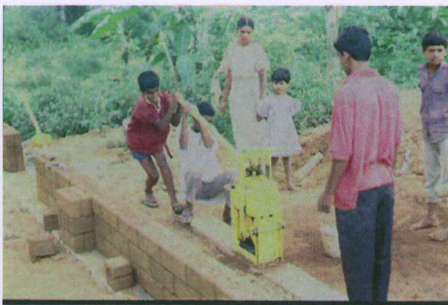
Figure 1. Cinva Ram Manual Machine
