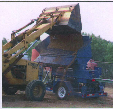
Figure 4. AECT 3000 Series Compressed Soil Block Machine
