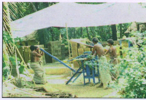
Figure 2. Auram Press Manual Machine
